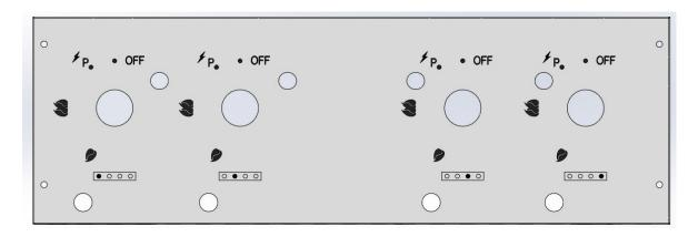
**OFF**: The burner and pilot will be shut off at this position.
