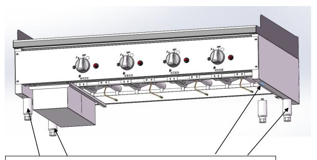
Find the four holes at the bottom of the frame ,screw in the legs firmly
