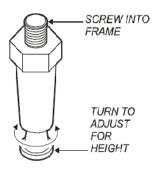
Verify that the unit sits firmly ON ALL FOUR LEGS. With the adjustable legs, adjust as required to level the appliance. All four legs must be adjusted to firmly contact the countertop in order to prevent tipping.
