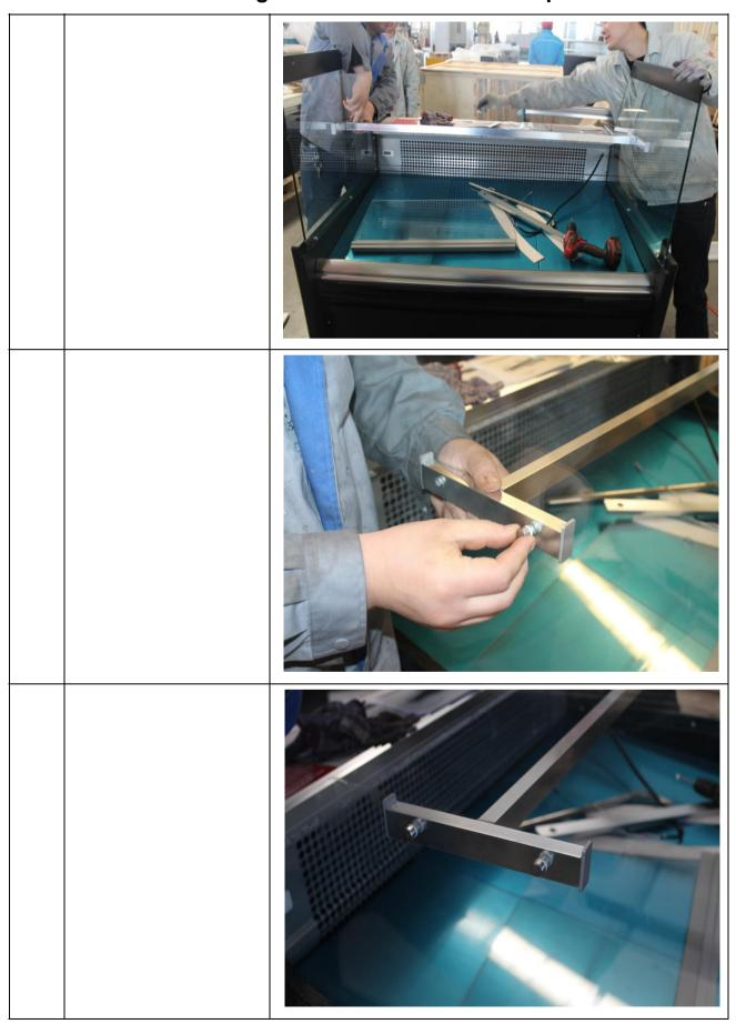
Install middle glass support for NSS1800FG, NSS2400FG Put the middle glass on the Step 5 support Install the top frame Step 6
